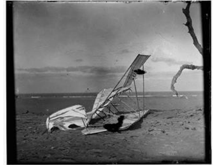
Crumpled glider wrecked by the wind on Hill of the Wreck, Wright Brothers, 1900.
